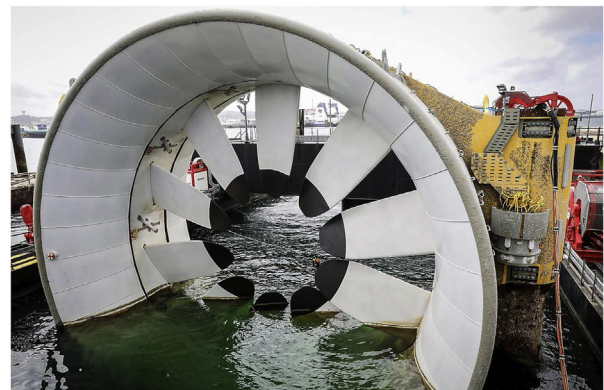
(b) 500 kW-rated turbine at the Paimpol Bréhat site in Northern France [12]
